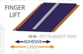
Customizable variations of release liner film, adhesives coat weights, slitting widths, number and type of reinforcements, and custom liner printing.
