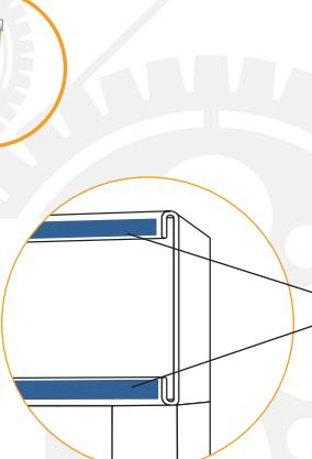
Use long length rolls for in-line taping on extrusions and on strip & spot applications
