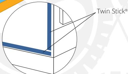
Foam tapes allow for greater surface contact on irregular surfaces. Firm, even pressure improves the bond.
